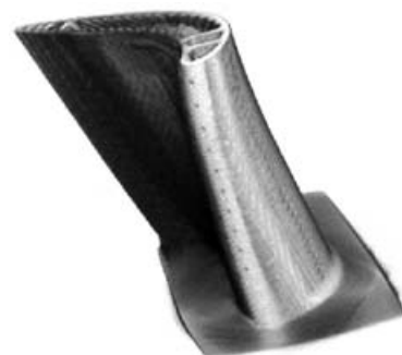
Fig. 4: Neutron tomographic reconstruction of a section of a coated Ni superalloy single crystal jet turbine blade.
